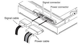
Each cable is keyed to ensure correct orientation. Seagate Laptop Thin SSHD SATA drives support latching SATA connectors.
